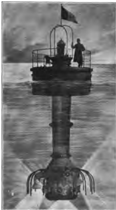
Hydroscope invented by Pino for exploring the sea bottom and successfully used in finding the galleons of Vigo Bay.
