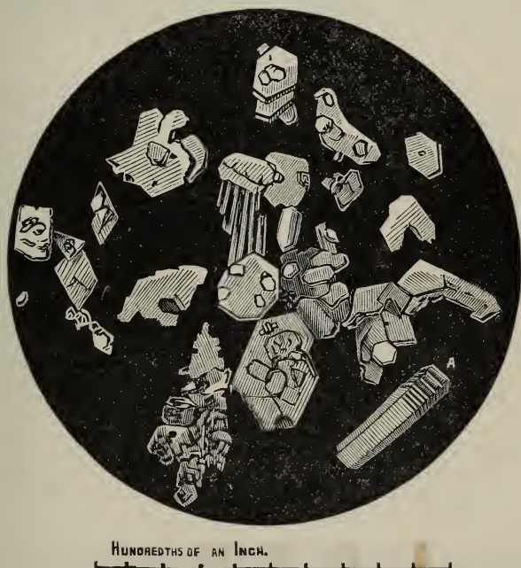
Fig. 12.—Boracic acid crystallized from solution, as seen under the microscope magnified 21 diameters. Drawn with the camera Lucida. (A) Rouleau of crystals.
